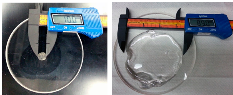
Figure 2. Digital photographs of 10 mm diameter pristine poly(IL) sample punched from the bulk (left); and the poly(IL) material fully swollen to ~89 mm diameter in DMSO (right).
